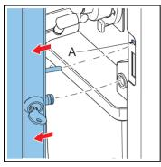
The door switch (A) automatically switches off the machine when the door is opened.
