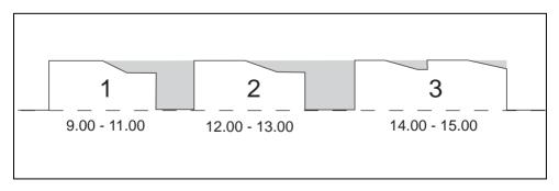
If the machine is switched on after being on standby and there is no dispensing, the machine will be in energy safe mode after 30 min. The temperature of the boiler drops every 30 min. with 5 °C. If there is dispensing after 2 hours the machine is reactivated. The machine uses less energy if there is no dispensing or is left switched on.
