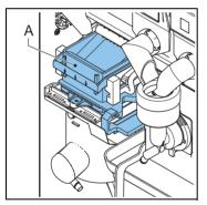
The brewer (A) receives the product from the canister. The product is made by vacuuming hot water through the filter. The brewer piston transfers the product to the outlet. A wiper transfers the residue to the waste bin.
