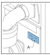
The on/off switch (A) puts the machine in the on/off position. The machine can still be charged after the machine is switched off. Unplug the machine to make sure that the machine is entirely uncharged.
