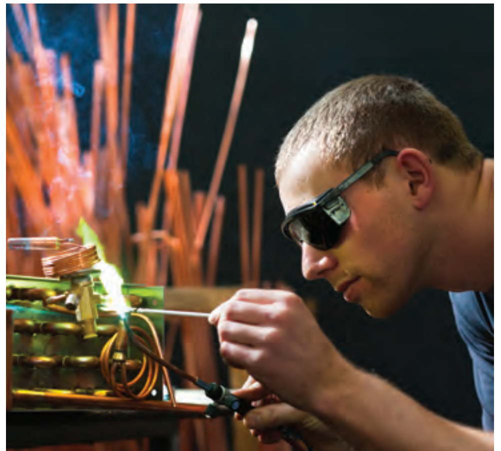
Soldering evaporator's elements
