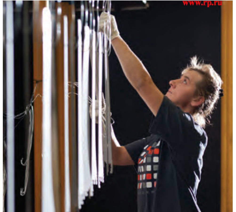
Preparing metal elements for painting
