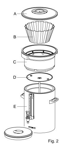
Attention! Always place the blender / transport disc and the lid when transporting the container by hand or serving trolly. This prevents spilling from the container.
